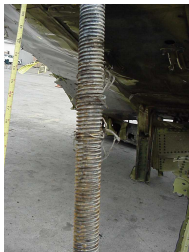
Figure: The jackscrew with acme nut threads [5].
