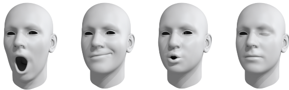
Figure 2: Examples of basic linear blendshape models. These blendshapes have been morphed to represent four common facial expressions (from left to right): a yawn, a smirk, a kiss, and a basic wink. [2]
