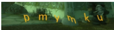
Figure 1: The Blizzard CAPTCHA makes use of a complex background in an effort to hide the text from automated processes while keeping the text recognizable to a human solver.
