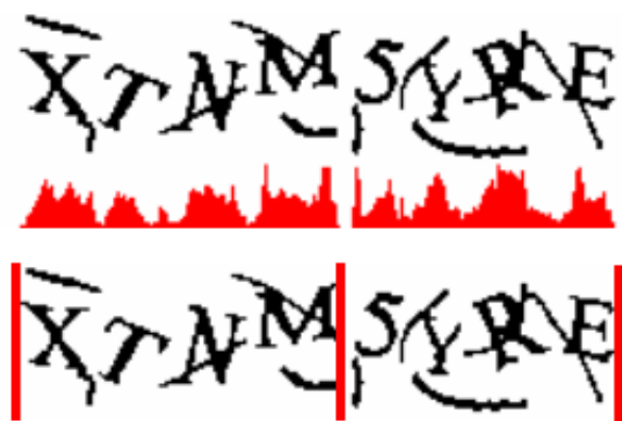
Figure 5: An example of histogram vertical segmentation with each bar representing the pixel count of the column directly above it in the top image. The long vertical lines in the bottom image represent segmentation breaks [7].
