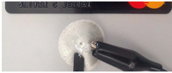
Figure 3: A small eavesdropping antenna [3] (card for scale)
