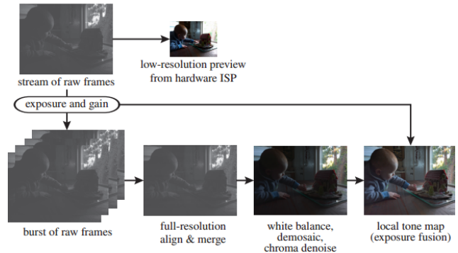
Figure 3: An overview of Hasinoff, et al’s., burst photography processing pipelines on the Nexus line of phones [4].
