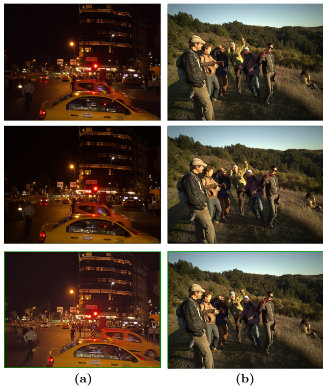
Figure 8: A comparison of two low-light photos produced by Hasinoff, et al.’s [4] burst merging (middle row) and Liu, et al.’s [7] pixel fusion (bottom row). Also, note that the green outlines indicate where cropping occurred within the pipeline. Taken from [5].
