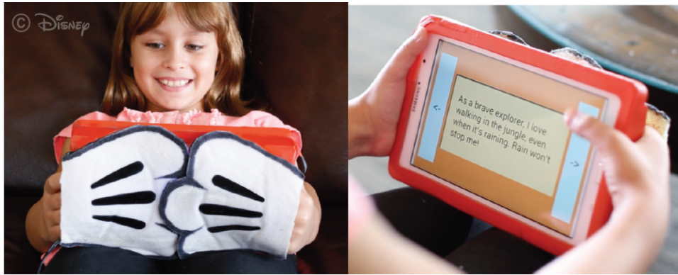
Figure 1: A child reading with FeelSleeve and feeling haptic effects associated with story events on her hands & a front view device. [7]
