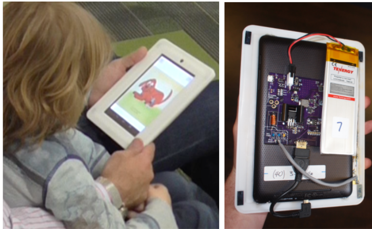
Figure 2: Left: TPAD Tablet device. Right: tablet mounted with circuit board, actuators, and battery (back cover removed). [6]
