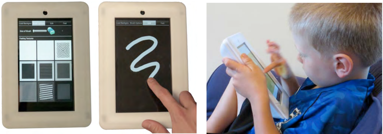
Figure 3: Left: Texture palette in e-book authoring application, users “paint” haptic patterns onto pages of an e-book, with black areas assigned high friction and white areas low friction. Right: Child (age 4) feels haptic textures on e-book pages [3]
