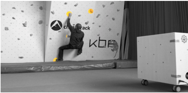
Figure 3: The betaCube unit placed in front of a climbing wall. Holds or grips are highlighted by the projector. [5]
