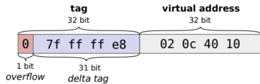
Figure 7: The first 32 bits are the tag which is added to the last 32 bits original pointer address. The very first bit is a overflow tag which determines whether the pointer is overflown or not. The following 31 bits are the Delta tag which represents the size of the buffer.
