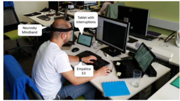
Figure 1: The participants in the study wore a headband and wristband that each contained the sensors used in the study. The tablet that caused interruptions is placed to the left of the participant’s main computer screen. [14]
