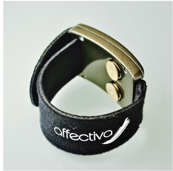
Figure 2: The Affectiva Inc. Q Sensor, which was the wristband used to sense EDA data in the interruption study by Goyal et al. [3]
