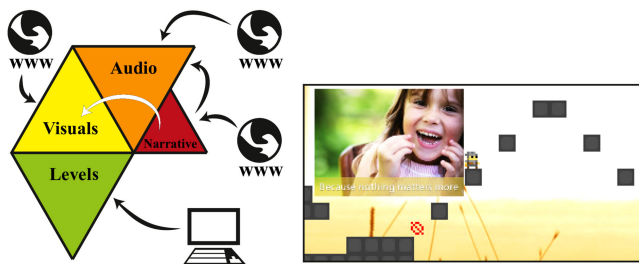
Figure 2. Facet orchestration diagram with in-game screenshot of Angelina with narrative, audio, and visuals being pulled from online sources. Arrows between facets indicate the influence of one facet's content on the generation of another's. Levels are procedurally generated, represented by the computer pointing to that facet. [7]
