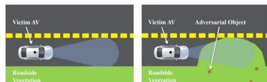
Figure 4. A vehicle/obstacle hiding attack scenario. With the placement of a few adversarial objects the parked car in front of the victim AV disappears from its sensors [8].
